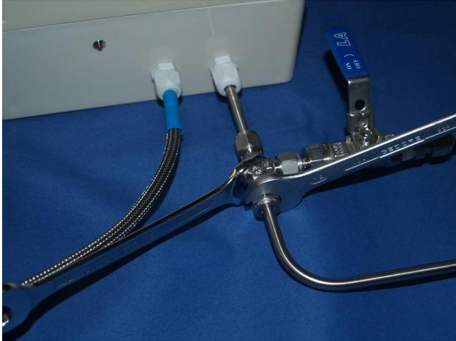
4. Apply pressure by opening the gas container valve and close again after some seconds.
